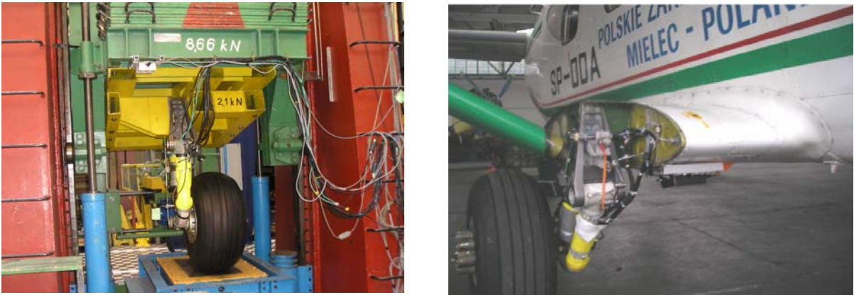
Fig.3 a) Test Bench in Institute of Aviation, Warsaw, Poland; b) field testing of Adaptive Landing Gear in PZL Mielec
